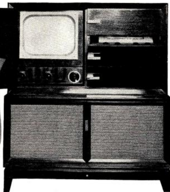
Fig. 1. RCA Model 730 TV2 after being converted to use a 14CP4 rectangular CR tube.
